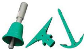
Detail of the finished, fettled castings
