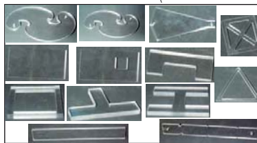
EFO-K2. Kit of Static Test Specimens (advanced kit)
