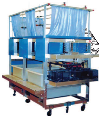
① Unit: ESHC(2x1 m). Hydrologic Systems, Rain Simulator and Irrigation Systems Unit (2x1 m).
