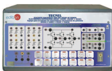
① Unit: TECNEL. Teaching Unit for the Study of Power Electronics (with IGBTs), including Control Interface. (Converters: DC/AC+AC/DC+DC/DC+AC/AC).
