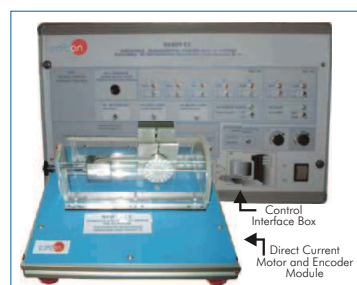
① Unit: SERIN/CC. Advanced Industrial Servosystems Trainer (DC motors)
