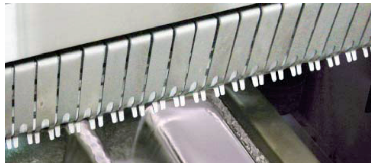
Dual Wave Option shown above - turbulent wave for SMD (optional) and laminar wave for through-hole soldering.
