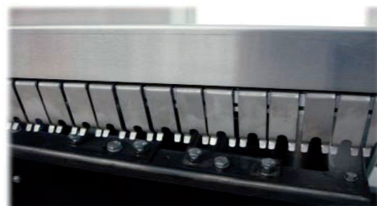
Finger conveyor for pallet or pallet-less operation.
