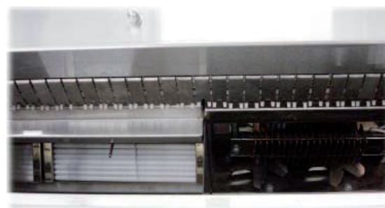
Independently controlled infrared and forced air convection preheaters compatible with VOC-free fluxes.
