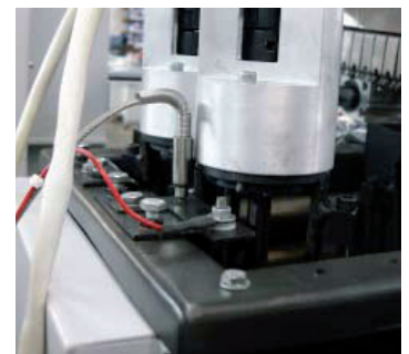
Solder level sensor with alarm
