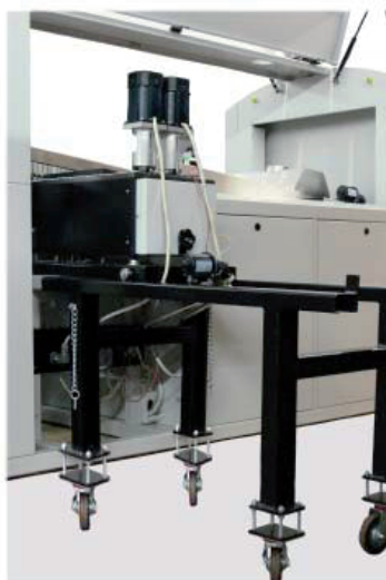
Motorized roll-out pot provides easy access.
