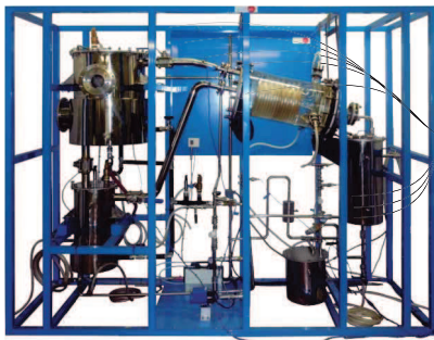
① Unit: QEDC. Batch Solvent Extraction and Desolventising Unit
