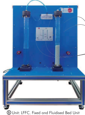
① Unit: LFFC. Fixed and Fluidised Bed Unit
