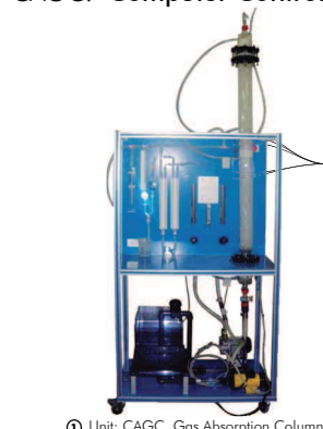
① Unit: CAGC. Gas Absorption Column
