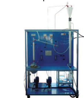
① Unit: UELL. Liquid-Liquid Extraction Unit
