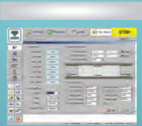
▲ Conveyor control interface display multiple parameters control, such as in/out direction, PCB width, X/Y/Z position.
