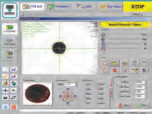
▲ Fiducial learning could be controlled by multiple parameter, such as shape, color, brightness, contract, etc. or completed automatically.
