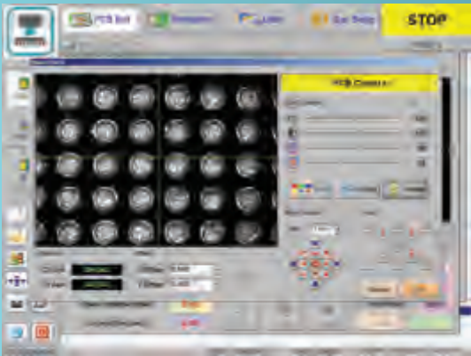
▲ 2D inspection function allow the inspection of short circuit, deviation and coverage rate of the solder paste.
